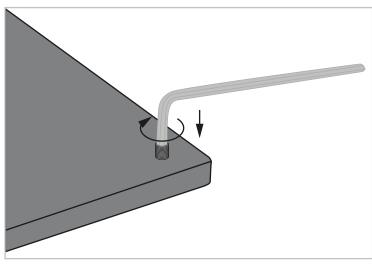
Screw in the adjustable foot flush-mounted from above with the supplied allen key.
