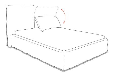
Due to a functional fitting both back parts are height-adjustable. To adjust the back, grasp it centrally and pull it up- or downwards in the desired position.
